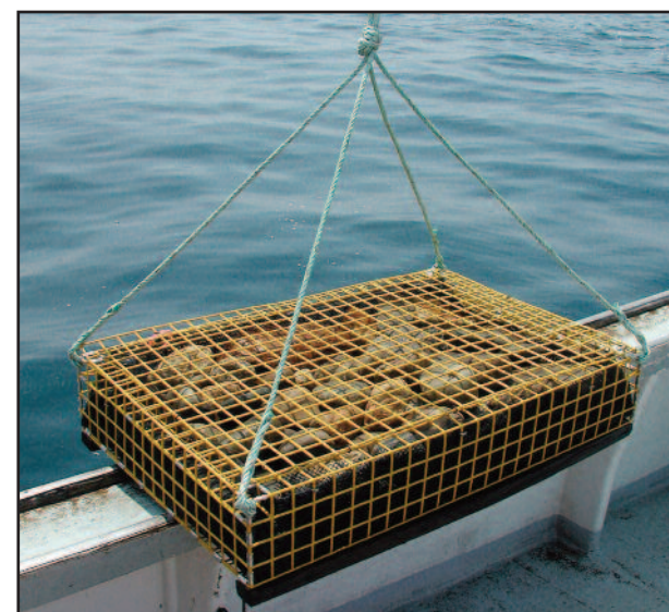
Passive postlarval collectors deployed with commercial trap hauling gear were developed in 2005 to expand the range and depth of the annual surveys to locations unsuitable for diving.
